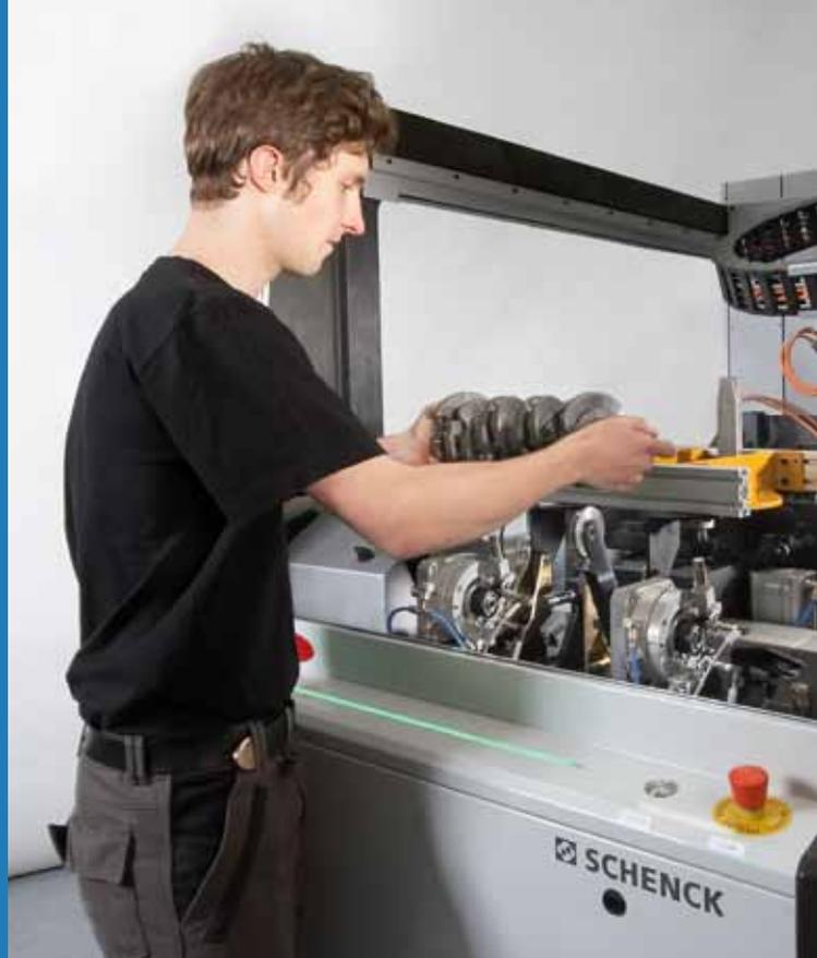
*Manual loading of a crankshaft*
